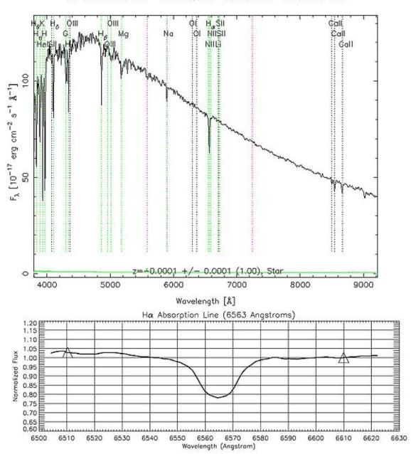
You saw in the table and graph above that the H $\alpha$  transition is at 6563 Ångstroms. So, the zoomed-in view shows the H $\alpha$  line for the spectrum. Does this star whose spectrum is shown here have more light at the H $\alpha$  wavelength, or less light? How do you know?
