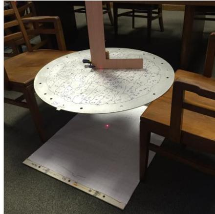
3. When the laser pointer is turned on, it should be pointing straight down towards the plate. This should ensure that if it points through one of the holes, it must be going straight through rather than at an angle.
