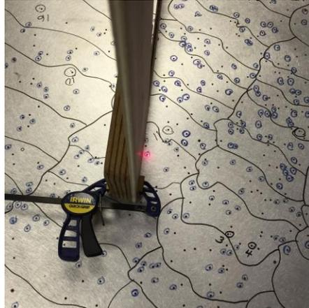
2. Attach a laser pointer to the top end of the T/L-square using rubber bands or something similar. The laser pointer should be attached so there is ample space between it and the plate. The small blocks can optionally be clamped on to the sides of the T/L-square so that it stays straight up-and-down.
